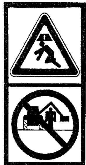
DO NOT WORK UNDER OR STAND UNDER UNSUPPORTED MACHINE
