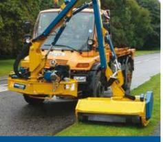
**Fitting kits for trucks** Shown fitted to Unimog U500.
